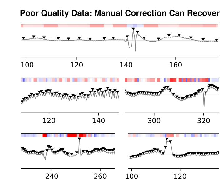
A faulty pulse oximeter was used for several subjects. physio\_calc was not designed to automatically detect these slower bumps, rather than sharper spikes. By inspecting data, it may be possible to tune the peak detection algorithm for atypical variations.
